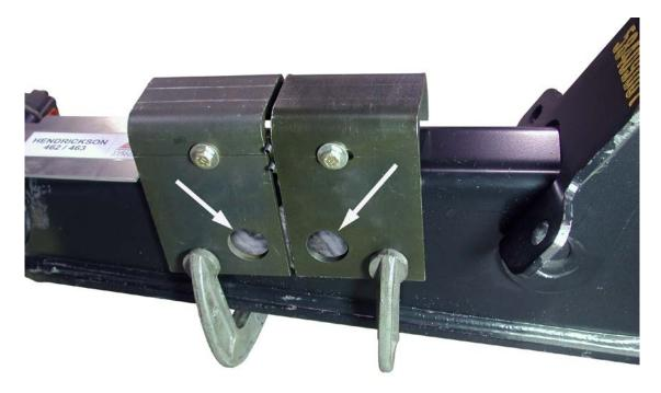
When the brackets have cooled, remove the clamps and angle fixture. The suspension beam is now ready for installation of the deflection sensor.
