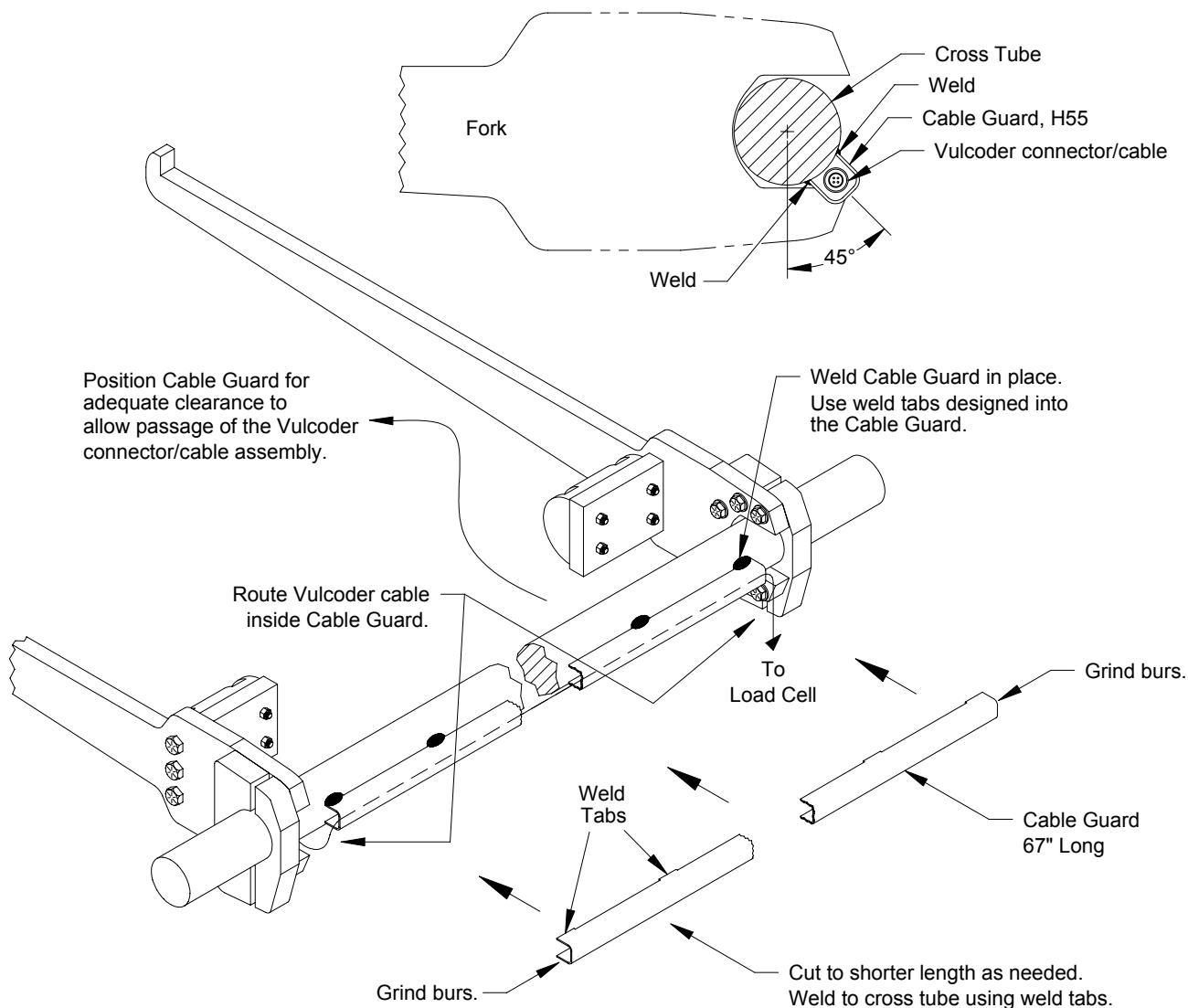
**NOTE:** After installation, paint using a rust preventative paint.
