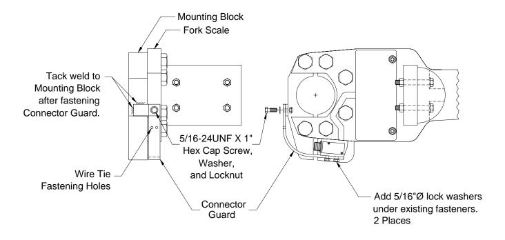
NOTE: After installation, paint parts using a rust preventative paint.
