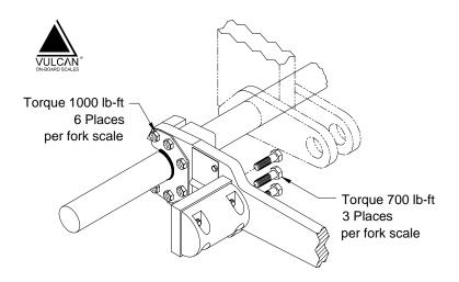
**NEW INSTALL:** Check Bolt Torque Once A Week For The First Two Weeks, Then Periodically When Truck Is Serviced. Painting And Undercoating the Front Fork Scales And Mounting Clamps Will Increase Their Service Life.
