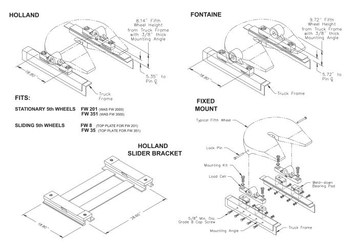
A system consists of two Vulcan Fifth Wheel Double Shear Beam Load Cells and two Fifth Wheel Mounting Kits containing load cell mounting bolts and weld-down bearing pads. An optional slide bracket is available for a Holland sliding fifth wheel.
