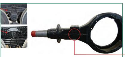
Side of Rear End Housing Welded
