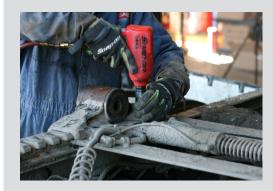
Lift Fifth Wheel Top Plate and Remove existing Brackets
