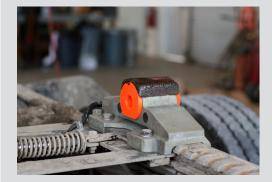
Place Holland ILS Load Cell on Slide Rail, Install 3 Cap Screw/Lock Washer Assemblies and Connect Vulcoder
